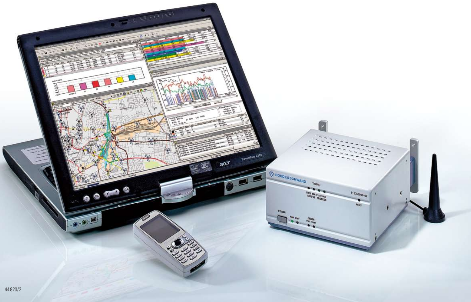
FIG 1 The R&S®TSMU automatically detects, analyzes and displays the results of co-channel and adjacent-channel interferences in GSM networks during a drive test.
