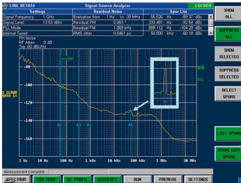
FIG 3 Typical measurement using the phase comparator method: Signal frequency, level and residual noise can be read off the display. The R&S®FSUP automatically detects unwanted interference, which can be blanked out. Spurious – including accurate frequency values – is listed in the display's top right corner.
