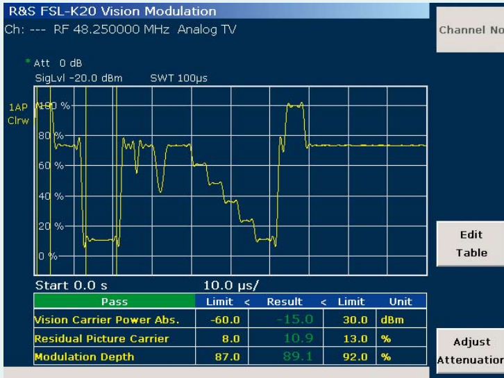
FIG 4 Vision modulation measurement of an analog TV signal.
