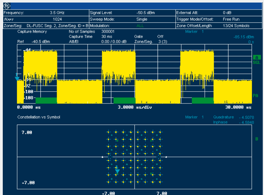
FIG 5 The upper part of the screen shows the recorded signal (power versus time). The lower part of the screen shows the constellation diagram. Since different bursts exhibit different modulation modes 64QAM, 16QAM and QPSK are displayed.
