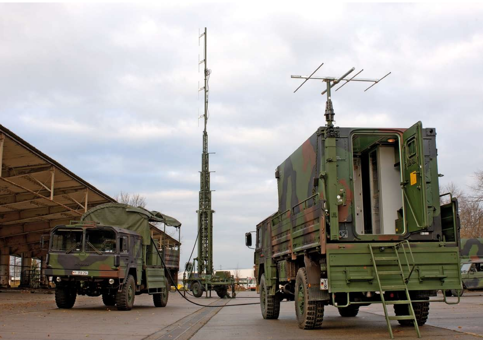
FIG 1 Mobile VHF FM broadcast transmitter system with setting-up unit (left), transmit antenna on the 25 m mobile antenna mast (center) and shelter (right).
