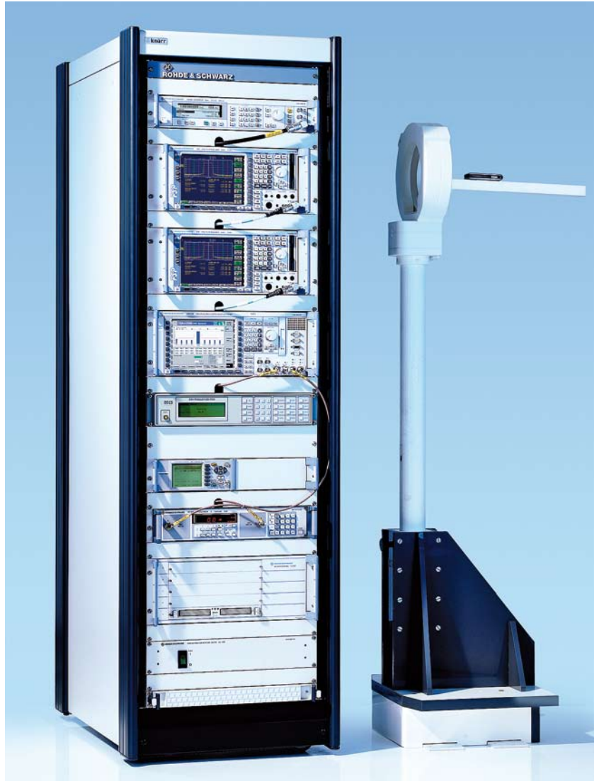
FIG 1 The RF Performance Test System R&S®TS9970 determines important RF characteristics of wireless communications equipment under realistic operating conditions.
